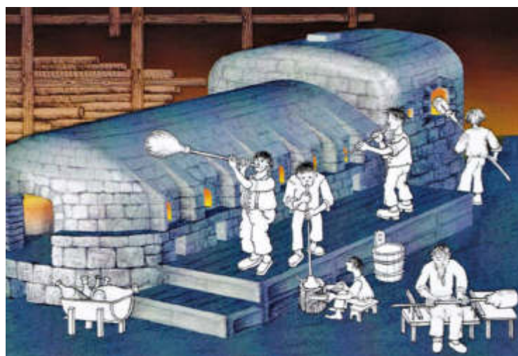
Glass melting furnace designed by Hans Greiner Print by Hans W. Schmidt
